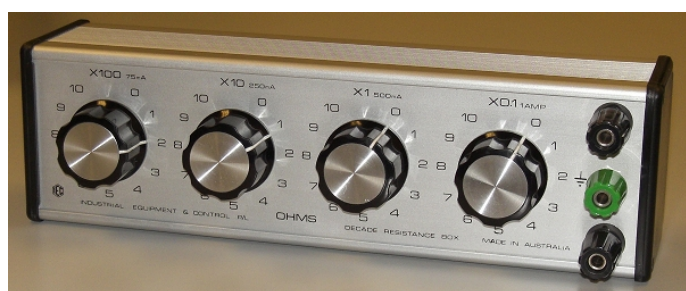
Figure 1: A typical resistor box used in laboratories [1].
