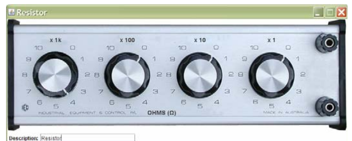
Figure 9: The GUI resembling the typical resistor box.
